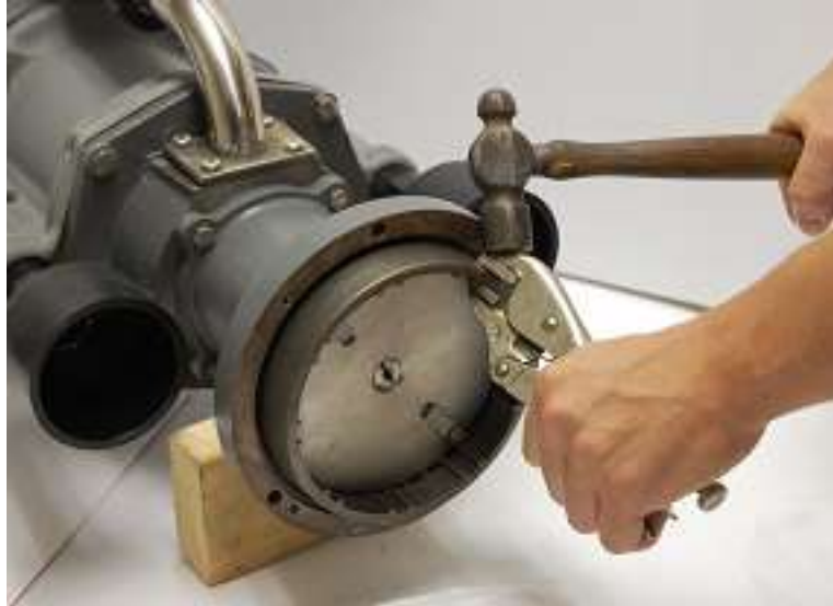
Figure 18 - Shredder Ring Removal
