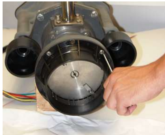
Figure 17 - Inlet Shroud Removal
