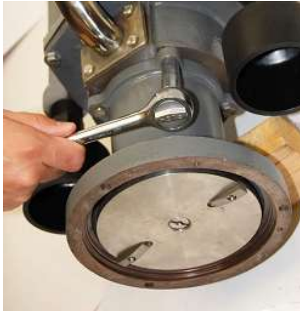
Figure 20 - Suction Housing Removal
