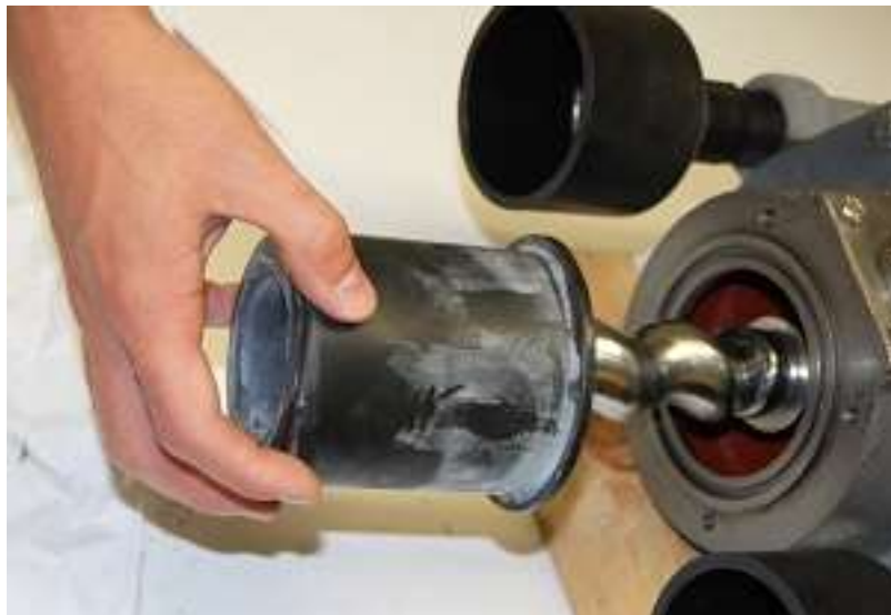
Figure 21 - Stator and Liner Removal
